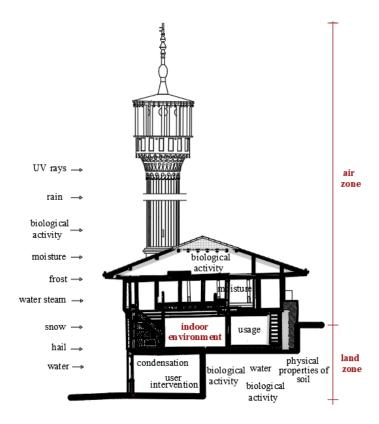
Figure 4. Factors causing deterioration of wood material
