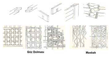
Figure 2. Local construction technique (eye stuffing, amulet stuffing and throat) (Özgüner, 1970)
