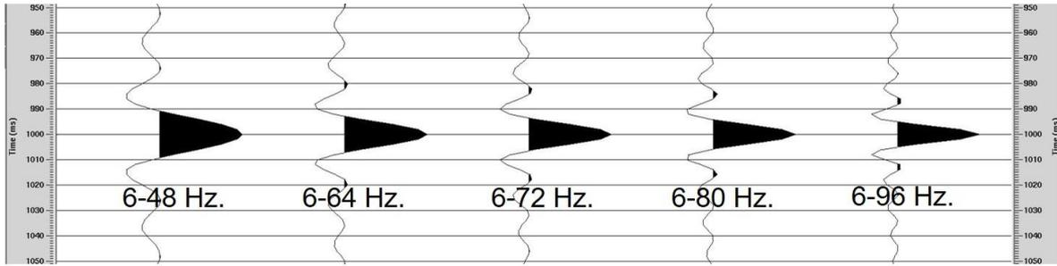
Figure 7a. Autocorrelation wavelets for different sweep bandwidth.
