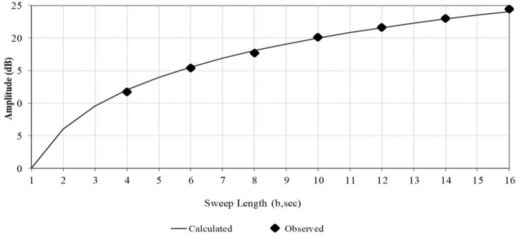
Figure 4b. Variation of peak amplitudes with sweep length.
