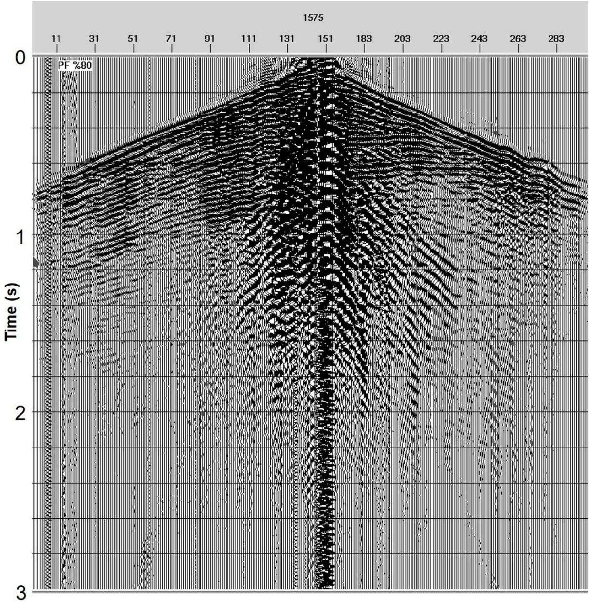
Figure 5d. 3D shot gather with 80% peak-force (Parameters are 12-64 Hz, 4 sweeps, 12 sec, Non-Linear -3 dB/Oct., 4 vibrators).
