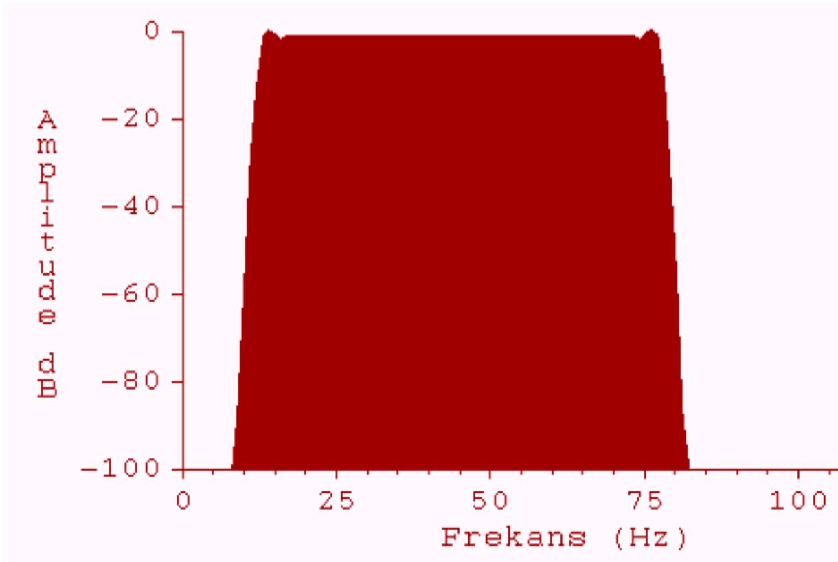
Figure 2c. Linear sweep in the frequency domain.
