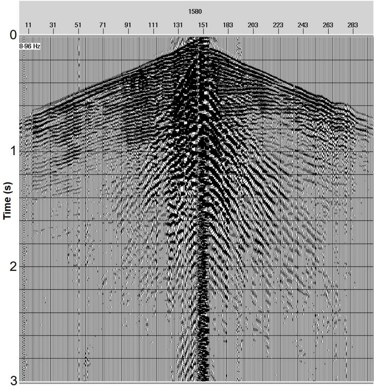
Figure 7d. 2D shot gather with wide bandwidth (Parameters are 8-96 Hz, 4 sweeps, 12 sec., Non-Linear -3 dB/Oct., Drive level 80%, 4 vibrators).
