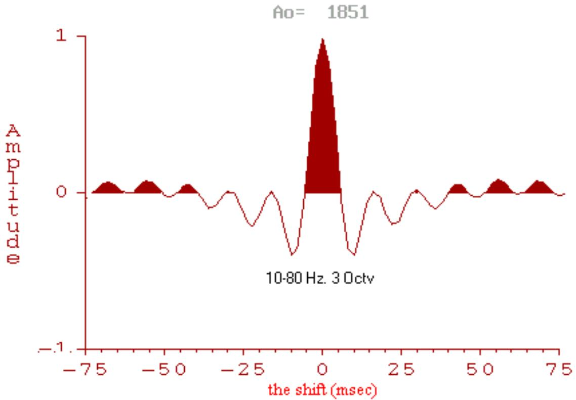
Figure 2d. Autocorrelation of sweep.
