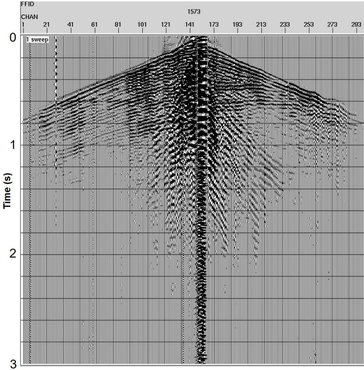
Figure 3c. 2D shot gather with 1 sweep (parameters are 12-64 Hz, 12 sec., Non-Linear -3 dB/Oct., Drive level 80%, 4 vibrators).
