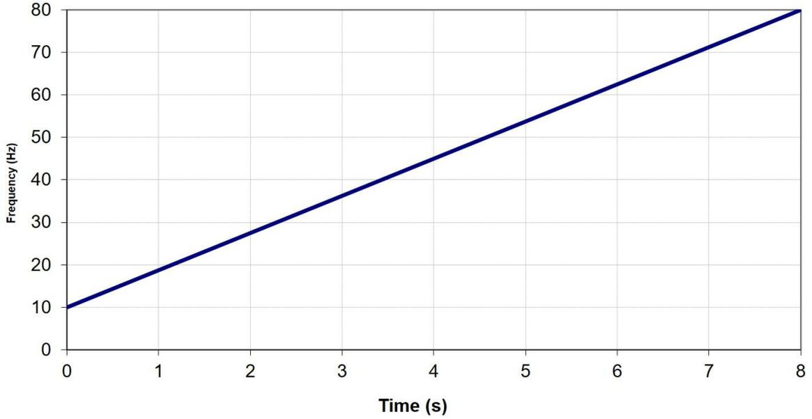
Figure 2a. Frequency-time relation of a linear sweep.
