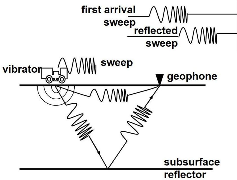
Figure 1b. Schematic view of vibroseismic technique (revised from Crawford et al., 1960; Seriff and Kim, 1970; Chapman et al., 1981 and Pann, 1986).
