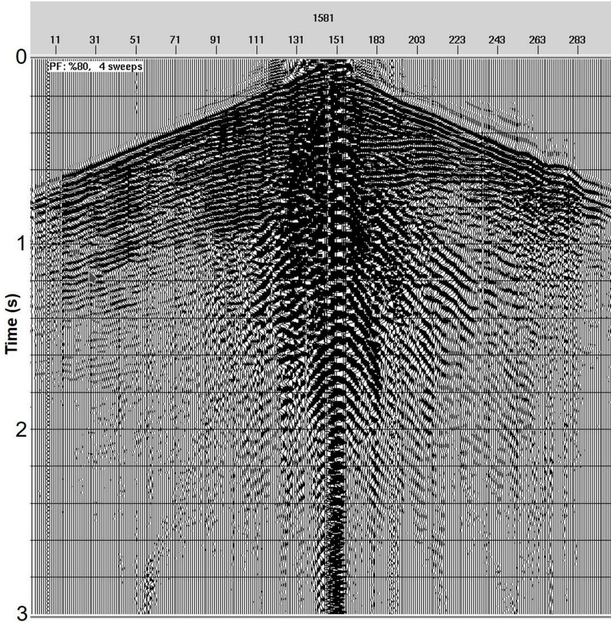
Figure 10b. 2D shot gather with Drive level 80% (High force) and 4 sweeps (Parameters are 12-64 Hz, 12 sec., Non-Linear -3 dB/Oct., 4 vibrators).
