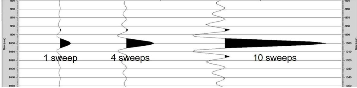
Figure 3a. Autocorrelation wavelets for different number of sweep.
