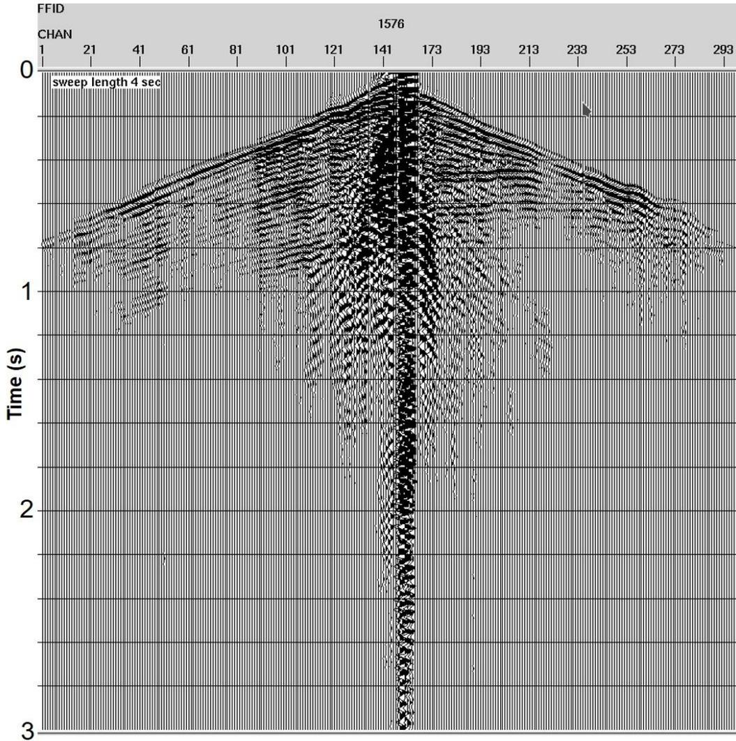
Figure 4c. 2D shot gather with 4 sec sweep length (Parameters are 12-64 Hz, 4 sweeps, Non-Linear -3 dB/Oct., Drive level 80%, 4 vibrators).
