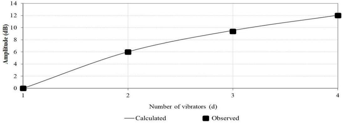
Figure 6b. Variation of peak amplitudes with number of vibrator.
