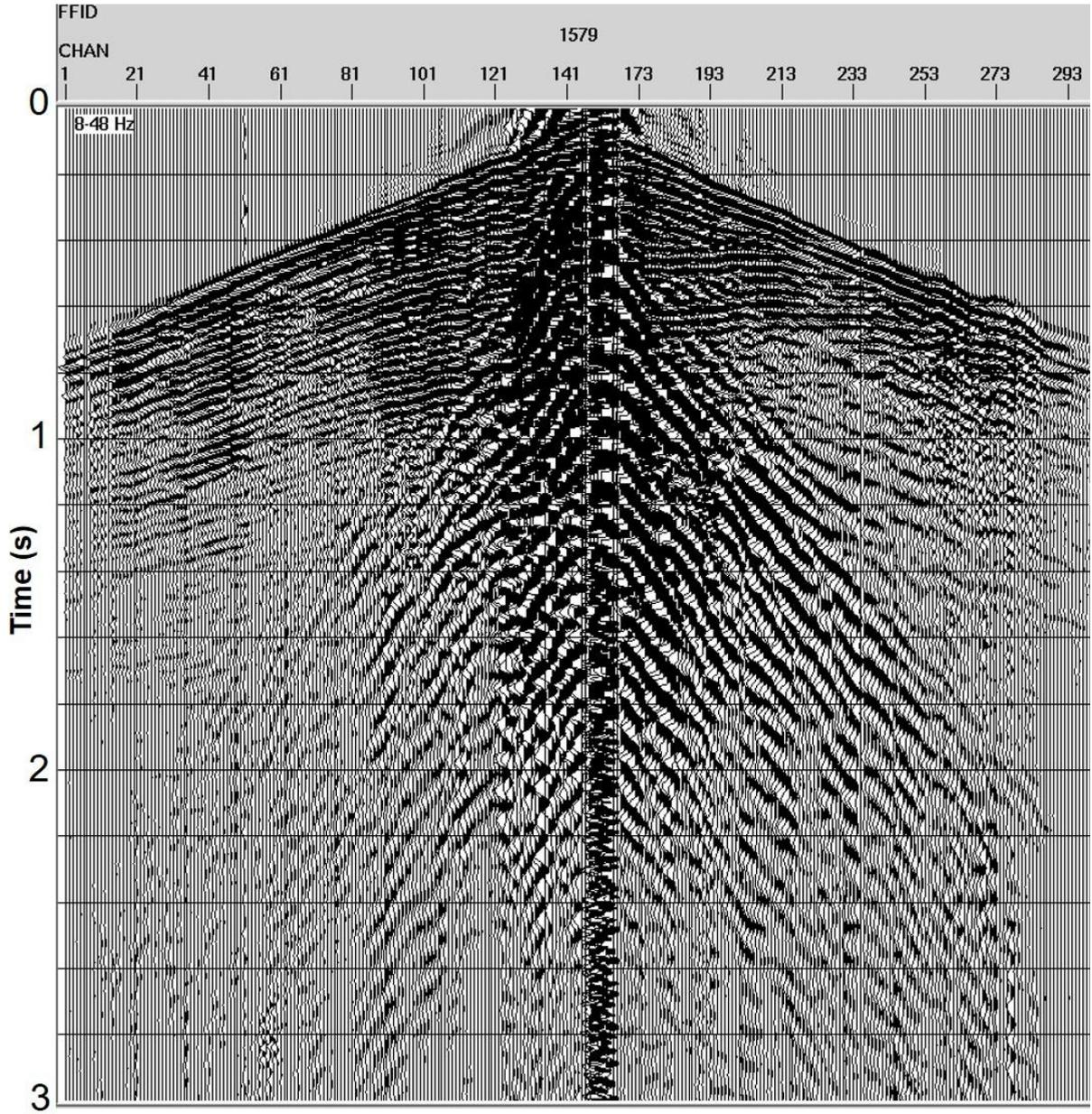
Figure 7c. 2D shot gather with narrow bandwidth (Parameters are 8-48 Hz, 4 sweeps, 12 sec., Non-Linear -3 dB/Oct., Drive level 80%, 4 vibrators).
