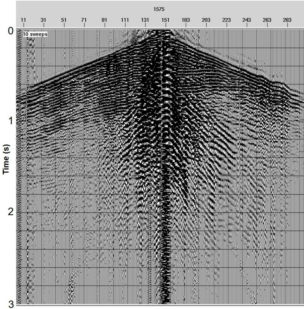
Figure 3d. 2D shot gather with 10 sweeps (parameters are 12-64 Hz, 12 sec., Non-Linear -3 dB/Oct., Drive level 80%, 4 vibrators).
