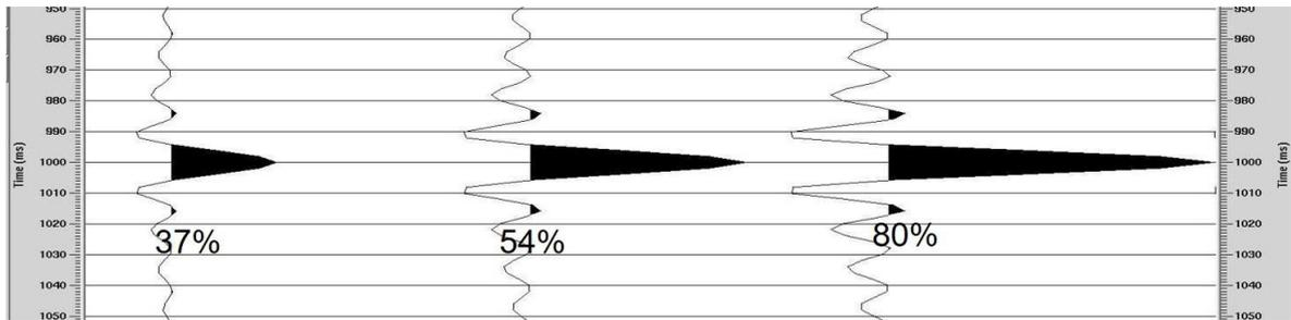
Figure 5a. Autocorrelation wavelets for different peak-force.
