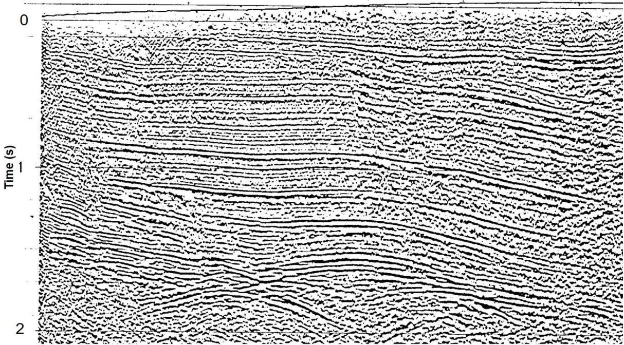
Figure 8a. Example of seismic section with 4 sweeps line-A (Parameters are 10-72 Hz, 8 sec., Linear, Drive level  $c=80\%$ , 4 vibrators).
