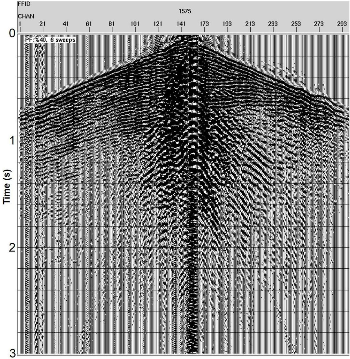
Figure 10a. 2D shot gather with Drive level 40% (Low force) and 6 sweeps (Parameters are 12-64 Hz, 12 sec., Non-Linear -3 dB/Oct., 4 vibrators).
