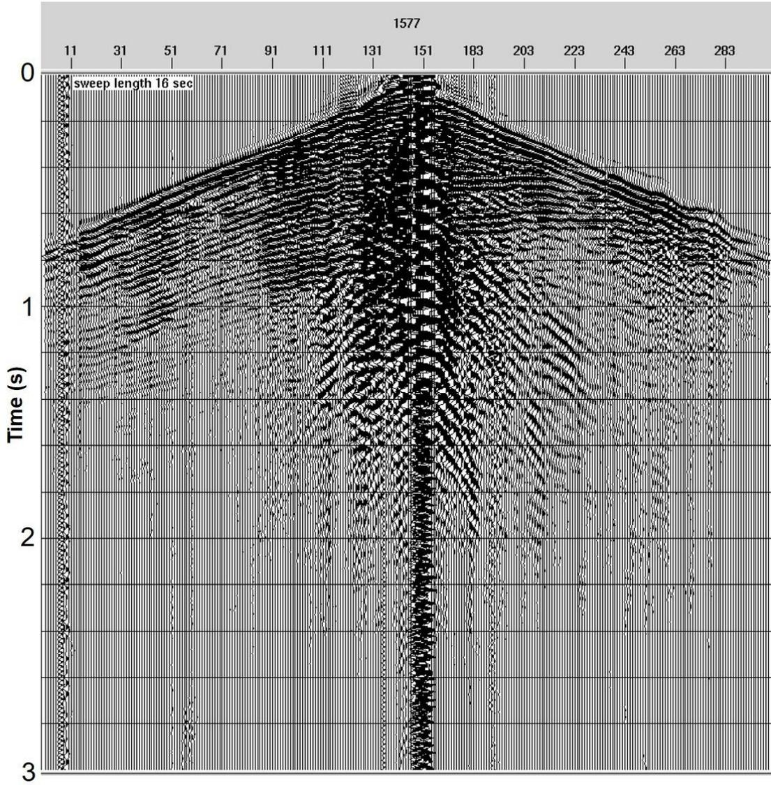
Figure 4d. 2D shot gather with 16 sec sweep length (Parameters are 12-64 Hz, 4 sweeps, Non-Linear -3 dB/Oct., Drive level 80%, 4 vibrators).
