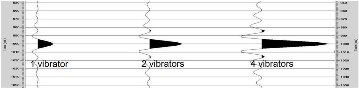
Figure 6a. Autocorrelation wavelets for different number of vibrator.
