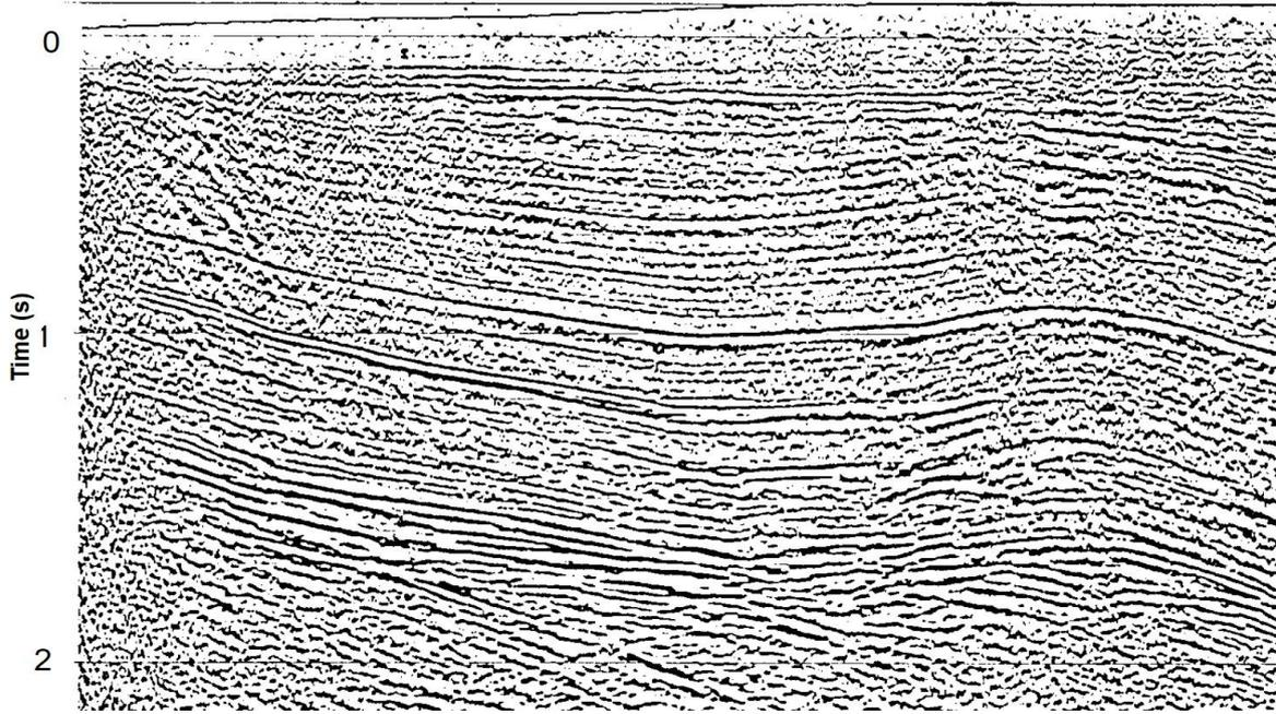
Figure 8b. Example of seismic section with 6 sweeps line-B (Parameters are 10-72 Hz, 8 sec., Linear, Drive level  $c=37\%$ , 4 vibrators).
