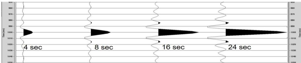
Figure 4a. Autocorrelation wavelets for different sweep length.
