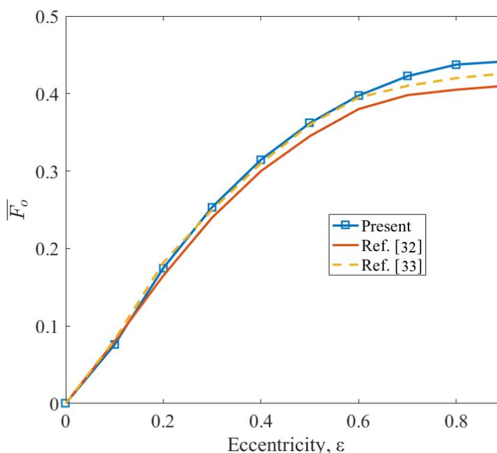
Figure 2. Variations of dimensionless fluid film forces with respect to eccentricity
