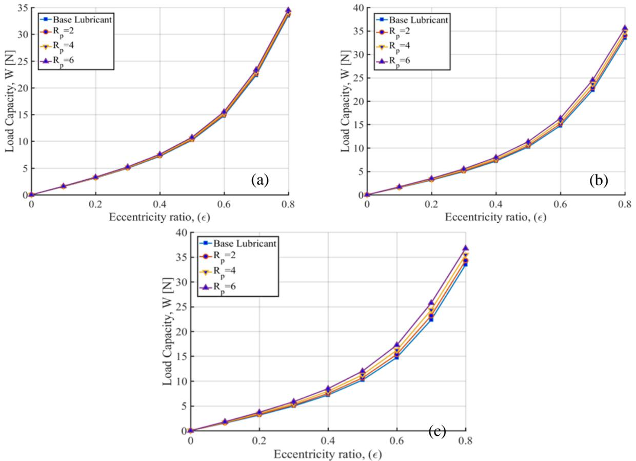
Fig. 3. Variations of the load capacity in regard to eccentricity ratio for different nanoparticle size, a)  $\phi=0.25\%$ , b)  $\phi=0.5\%$ , c)  $\phi=0.75\%$
