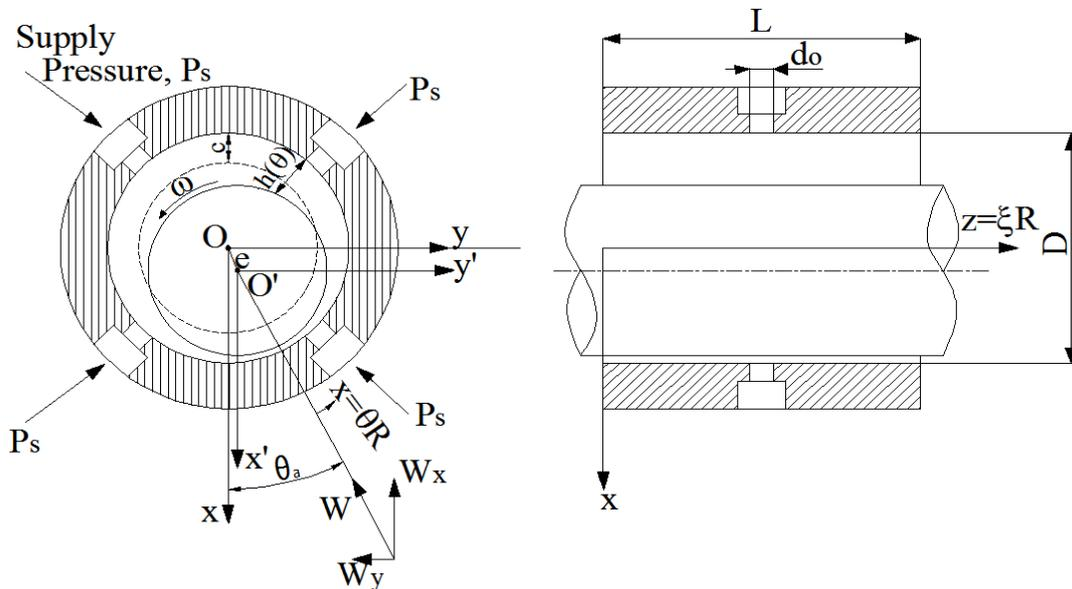
Figure 1. A hydrostatic journal bearing [28]
