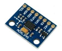
Figure 3. ADXL 345 triaxial accelerometer
