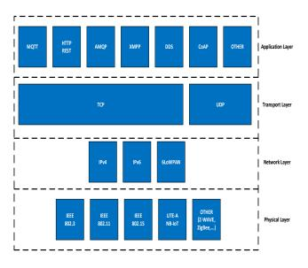
Figure 3. Communication Layers
