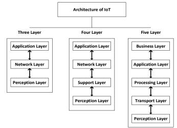
Figure 4. IoT Layer Architecture
