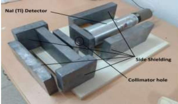
Figure 2. The picture of the experimental setup [9]
