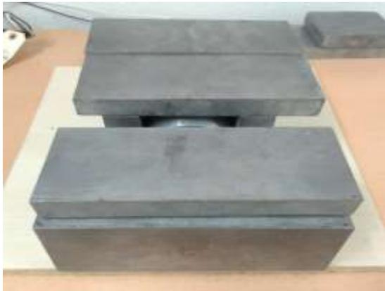
Figure 3. Side and up shielding plate
