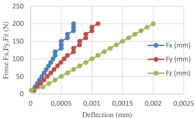
**Figure 3.** Force-deflection curve for  $F_x, F_y, F_z$
