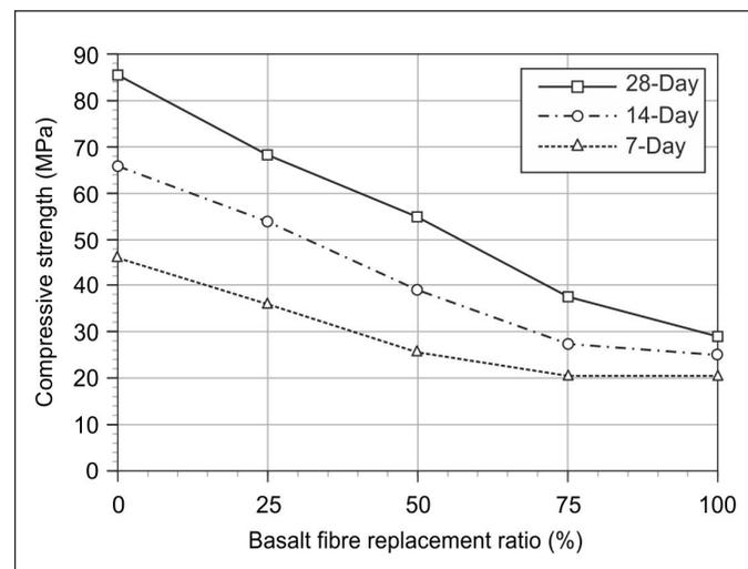
**Figure 4.** The variation of compressive strength values in terms of the basalt fibre replacement ratios.
