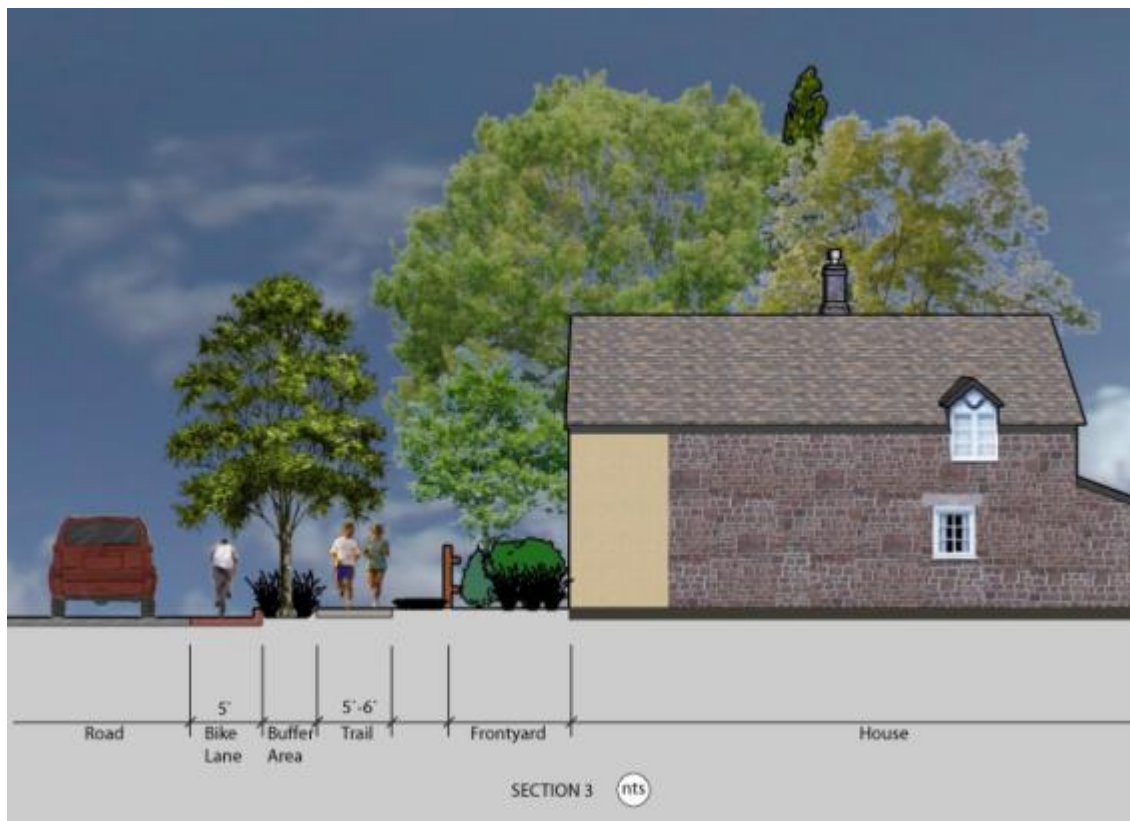
Figure 9. The shared-use trail designated to be shared by existing vehicular traffic with proposed bicycle and other non-motorized uses.
