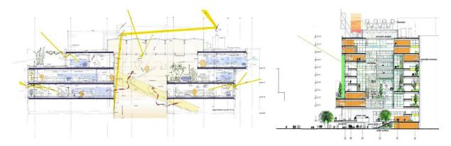
Figure 4. Roof mounted heliostats and section, Genzyme Center [11]
