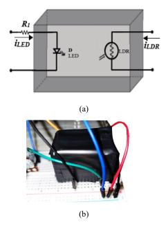
*Fig. 3. a) The topology and the circuit of the optocoupler and b) the external view of the optocoupler box made.*
