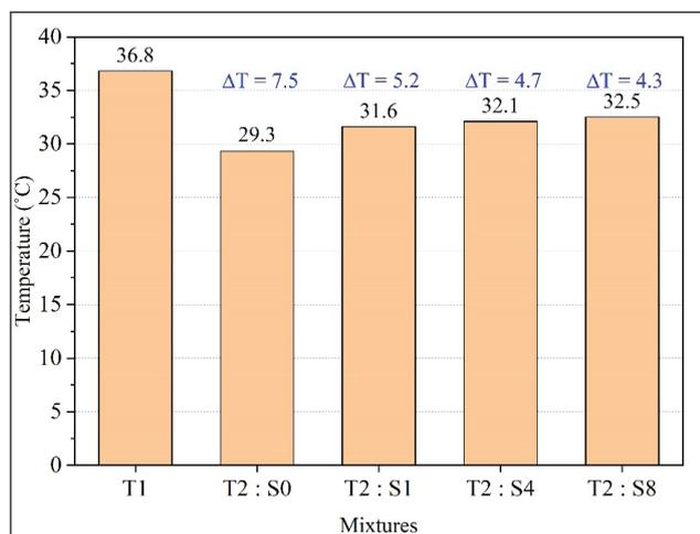
Figure 14. T<sub>2</sub> temperature change of S0, S1, S4 and S8 screeds versus T<sub>1</sub> temperature change at T<sub>w</sub> is maximum.
