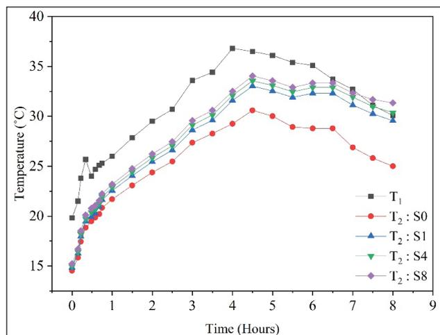
Figure 13. T<sub>2</sub> temperature change of S0, S1, S4 and S8 screeds versus T<sub>1</sub> temperature change over time.
