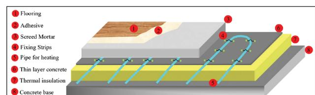
Figure 2. Detailed view of underfloor heating systems.
