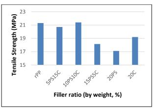
Figure 2. Tensile strength properties of composites materials
