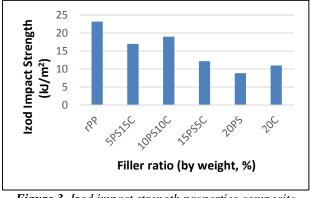
Figure 3. Izod impact strength properties composite samples
