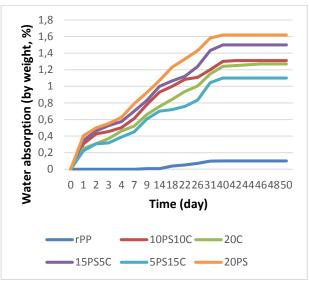
Figure 5. Water absorption properties of composites samples
