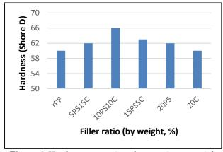
Figure 4. Hardness properties of composites materials
