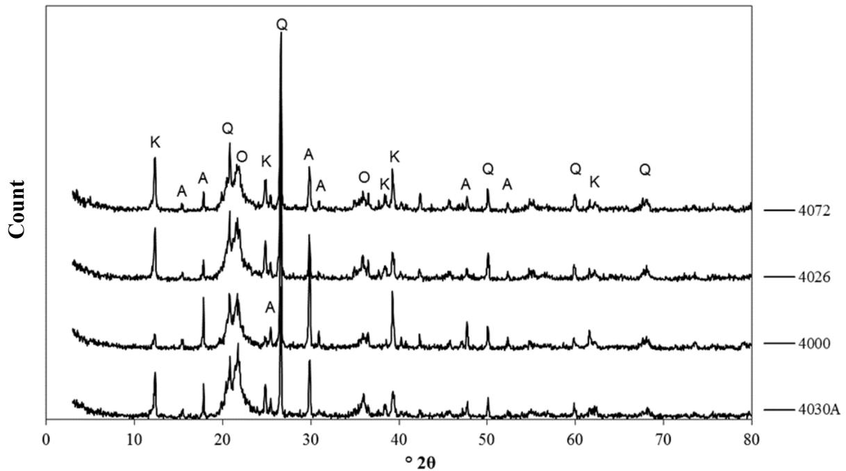
**Figure 2.** XRD graphs of raw samples (K: kaolin; Q: quartz; A: alunite; O: opal)
