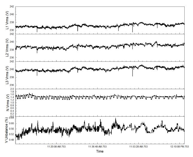
**Figure 7.** Time-dependent voltage values for all three phases and the neutral line, along with the voltage imbalance in the system.
