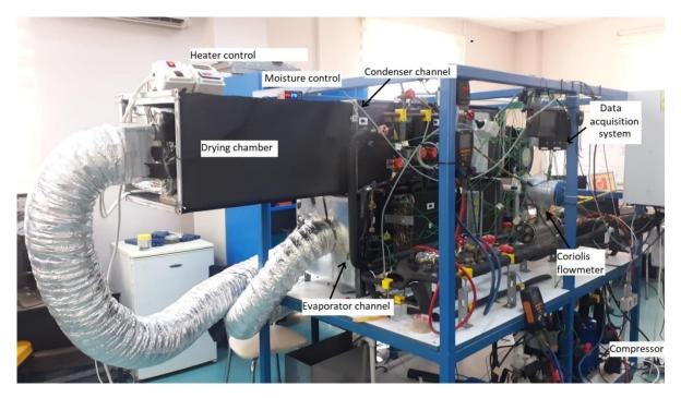
Figure 1. The heat pump drying system
