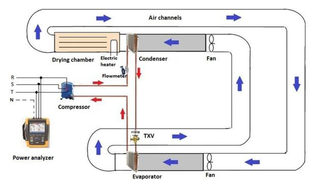
Figure 2. Paths followed by refrigerant flow and airflow in the HPD system
