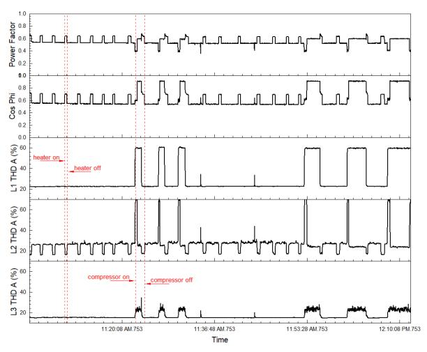
Figure 6. A graph illustrating the impact of harmonics on power factor.
