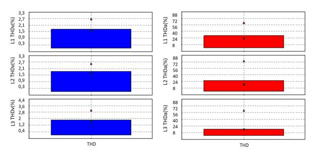
Figure 5. Histogram graph showing voltage and current harmonics for each phase.
