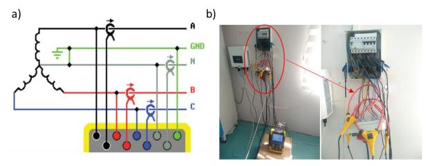
**Figure 3.** a) connection diagram of the probes to the three-phase system b) real image of the installation of the measurement setup into the system
