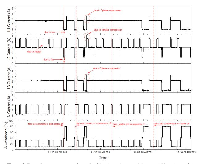
**Figure 8**. Time-dependent current for each of the three phases and the neutral line, along with the graph showing current imbalance in the system.
