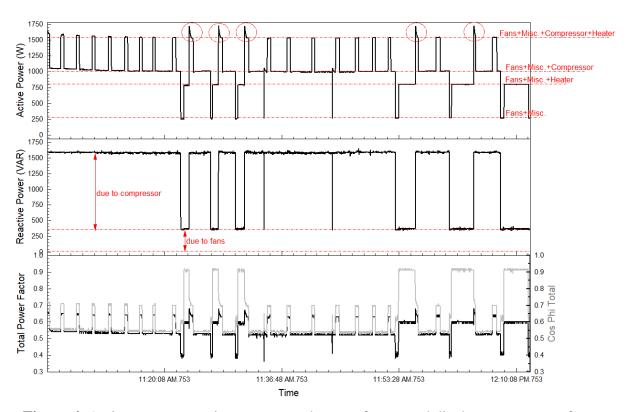
**Figure 4.** Active power, reactive power, total power factor, and displacement power factor values drawn by the HPD system.
