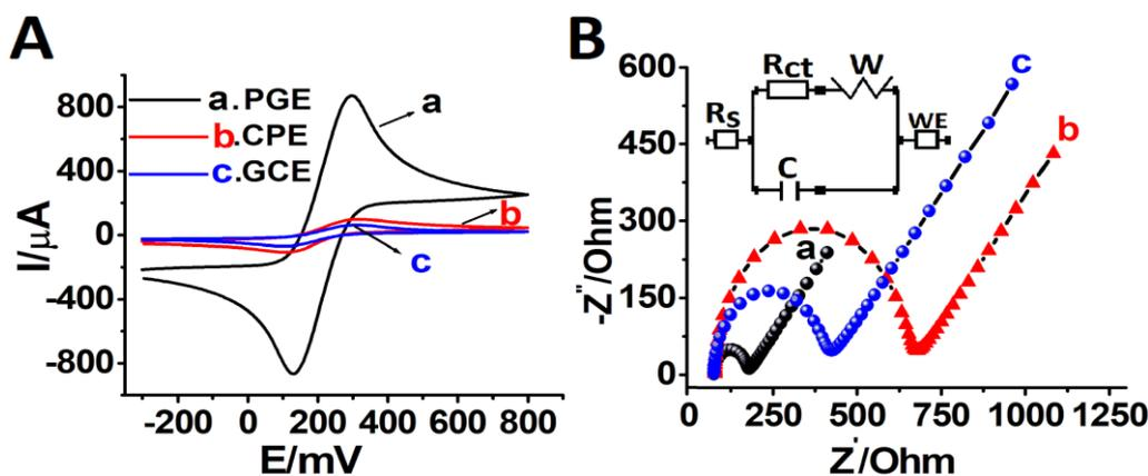
**Figure 2.** A) CVs and B) EI curves for 5.0 mM of  $\text{Fe}(\text{CN})_6^{3-/4-}$  solution contains 0.10 M KCl at (a) PGE, (b) CPE, and (c) GCE, the inset of Figure B is the electrochemical impedance circuit model: (C: Capacitance for double-layer;  $R_s$ : Ohmic resistance; WE: Working electrode ; W: Warburg impedance, (Scan rate (S.rate): 50 mV/s)
