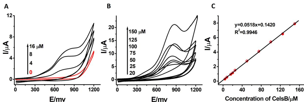
**Figure 6.** A) CVs from 0 to 16  $\mu\text{M}$  CelsB B) CVs from 20  $\mu\text{M}$  to 150  $\mu\text{M}$  CelsB (BRBS pH5.0; S. rate: 50 mV/s ) C) Calibration curve of CVs acquired from CelsB at increasing concentrations
