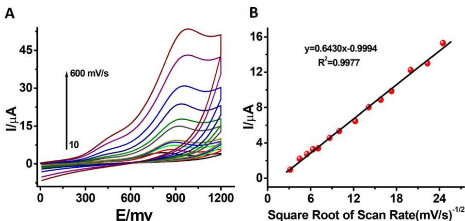
**Figure 5.** A) CV responses acquired from PGE against 50  $\mu$ M CelsB at different S.rate (10-600 mV/s) at pH 5 (BRBS) potential range: 0 – 1200 mV, B) the linear variation of the square root of the scan rate versus the oxidation peak currents of CelsB
