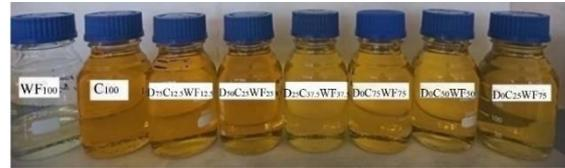
**Figure 5.** Prepared Biodiesels and Fuel Blends
