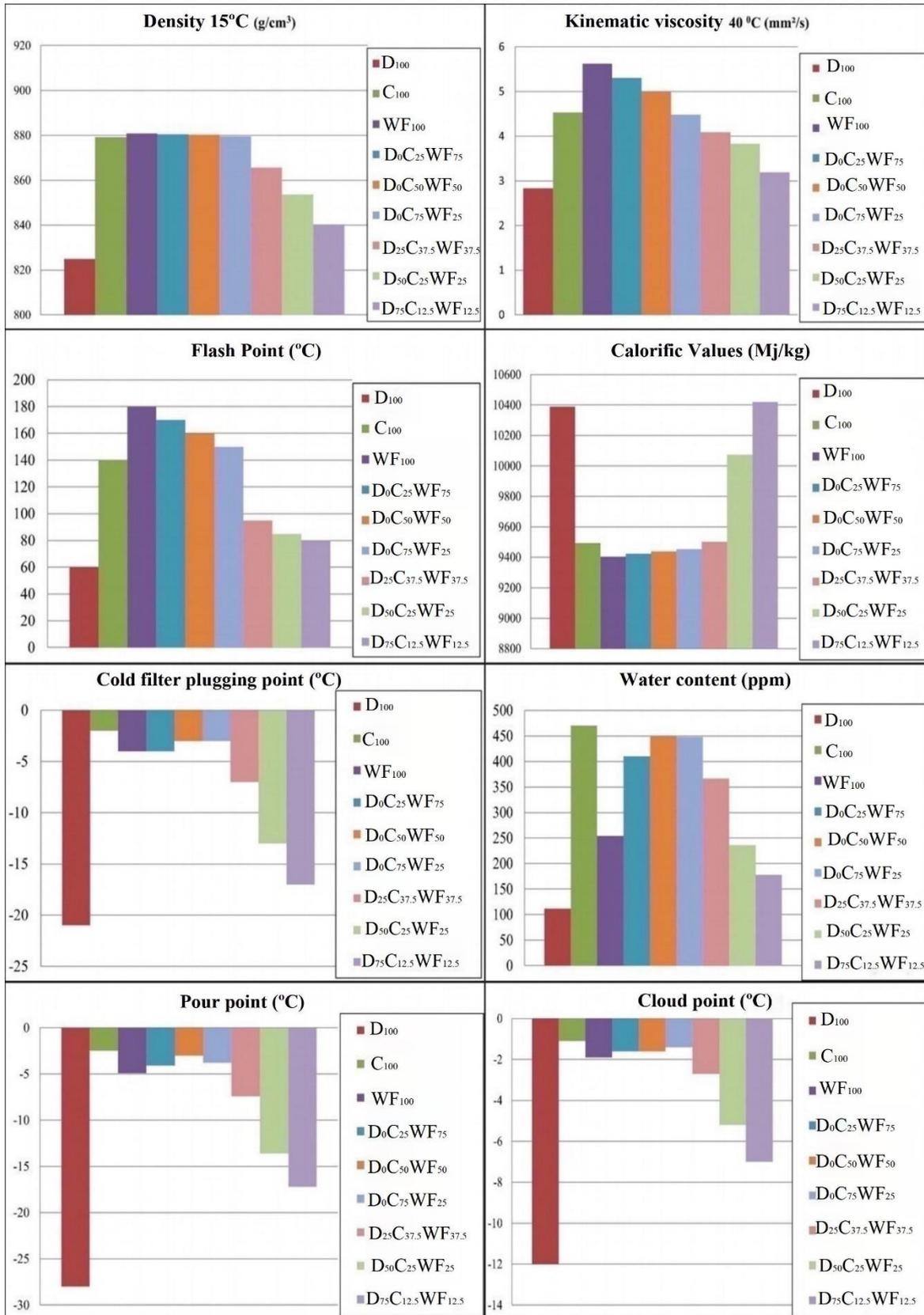
Figure 7. Fuel properties of diesel, camelina biodiesel, waste cooking oil biodiesel, binary biodiesel, and binary biodiesel+diesel blends.
