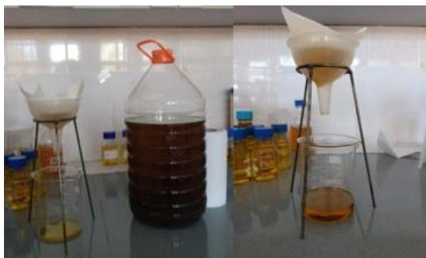
Figure 2. Filtration process applied to raw camelina and waste frying oils.
