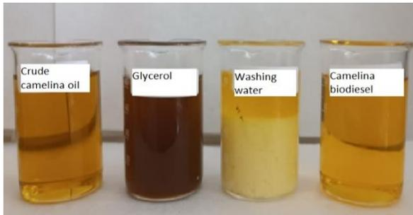
**Figure 4.** Stages of Camelina Biodiesel Production Using the Transesterification Method.
