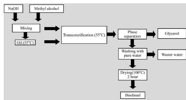
Figure 3. Stages of Biodiesel Production [15-1].
