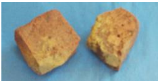
Figure 10. Appearance of the brick sample after Na 2 SO 4 solution attack.
