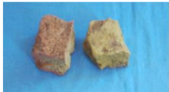
Figure 11. Appearance of the brick sample in relation to NaCl solution.
