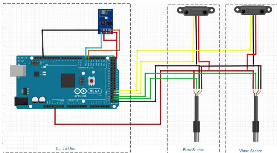
**Figure 2.** System control unit circuit diagram.
