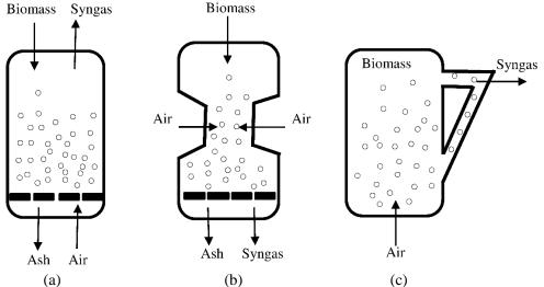
Fig.1. Different gasification technologies (a) updraft, (b) downdraft, (c) circulating fluidized bed (CFB)
