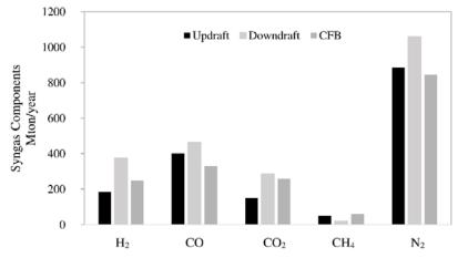
Fig.2. Production rate of different syngas components from updraft, downdraft and CFB systems
