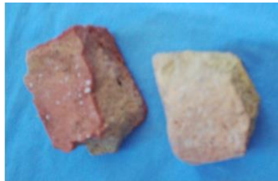
Figure 9. The efflorescence after bricks interaction with H 2 SO solution.
